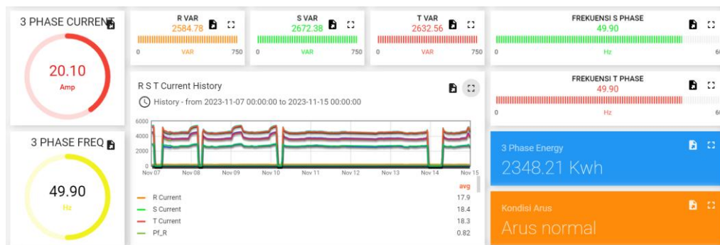
Figure 2. Dashboard of Smart Real-Time Motor Control Center
