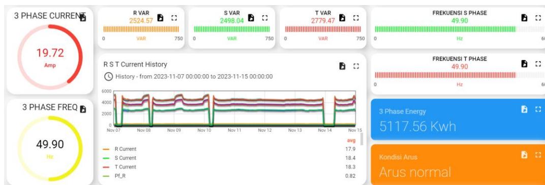
Figure 7. Notification regarding current conditions on the 88BT Motor GT 1.2
